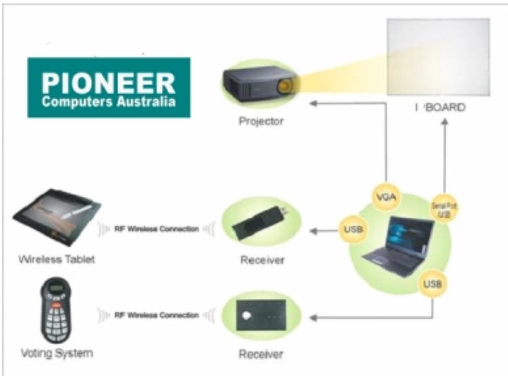
Basically, the whole system consists of four necessary components: **iBoard**, driver software for **iBoard**, desktop or laptop and projector. The software for **iBoard** is provided free if the board is purchased and it should be installed first before the operation of **iBoard**.
